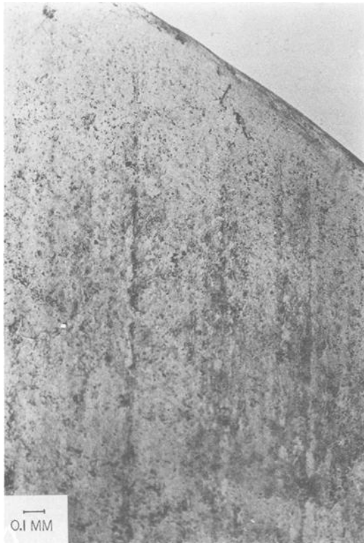
FIG. 3—Thinned nail specimen viewed between crossed polarizing filters.
